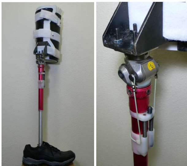
(a) Final prototype (b) Prosthetic knee joint Fig. 6. The final prototype, TAMC2
