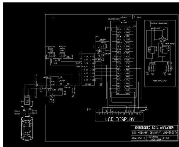
Fig.4: Schematic Diagram of Embedded Soil Analyzer
