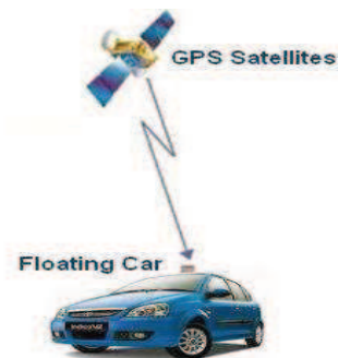
Fig. 2 A moving vehicle (Floating car) fixed with a GPS receiver
