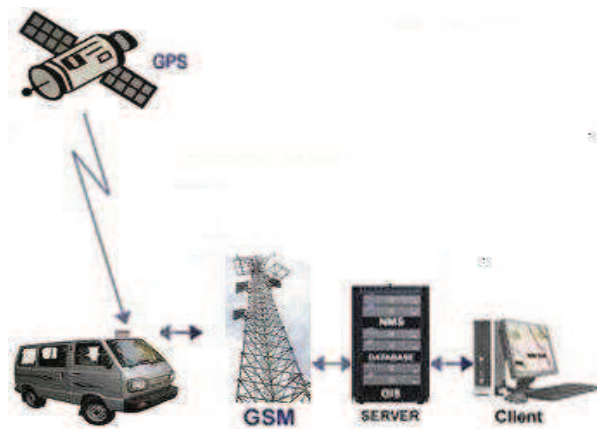
Fig. 1 GPS tracking with the help of a GPS receiver fixed in a moving object.
