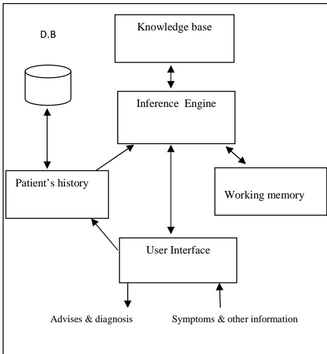
Fig. 1. Structure of the system
