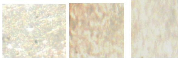
**Fig: 3.4.4 Aluminium (sintering temp=400°C); Aluminium (sintering temp=420°C) & Aluminium (sintering temp=430°C)**
