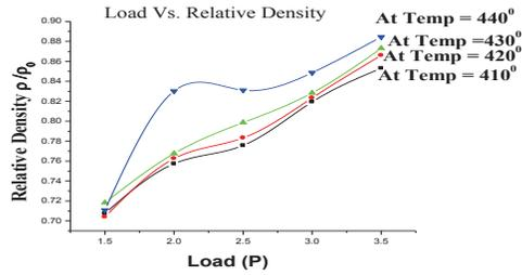
**Fig.- 3.1.2 Variation between load in tone and relative density**
