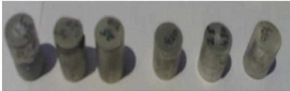
**Fig.-2.6 compacted billets of aluminium**
