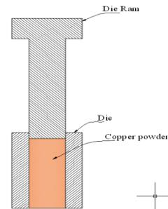
**Fig.2.3 Filling of copper powder material**
