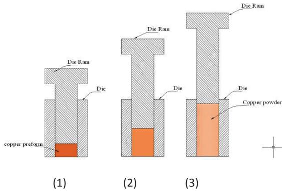
**Fig.2.4 Compaction process on Hydraulic press and UTM**
