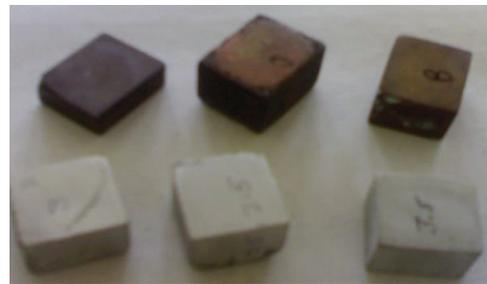
**Fig.-2.10 Rectangular Sintered billets of copper & aluminium powder**
