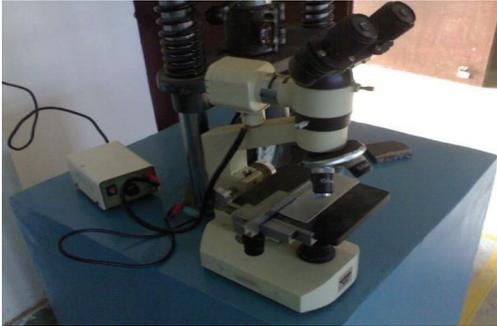
Fig. 2.17 Metallurgical Microscope
